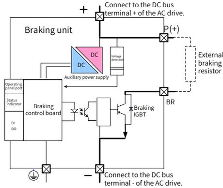
Figure 1-2 Braking unit application principle
