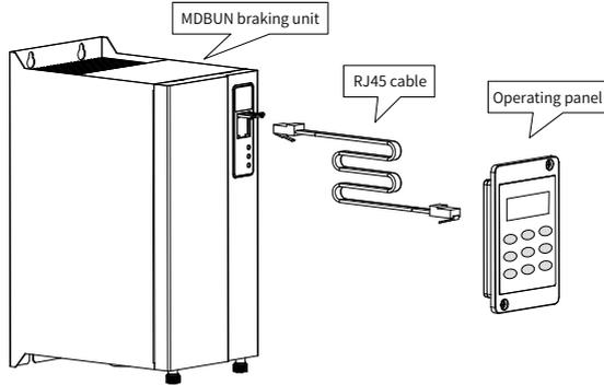
Figure 3-2 Wiring between the external operating panel and the braking unit
