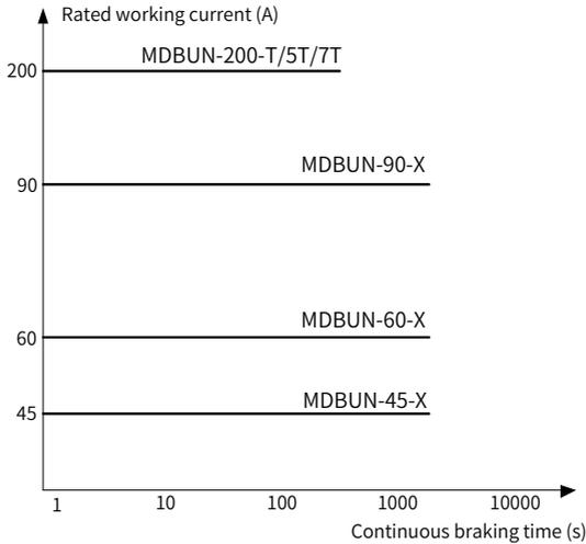
Figure 1-3 Load curve of the MDBUN series braking unit
