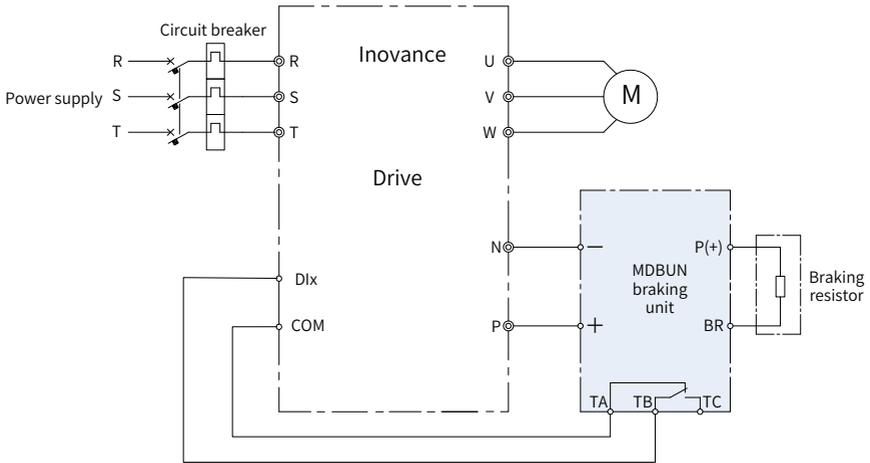
Figure 2-8 Standard wiring method 2
