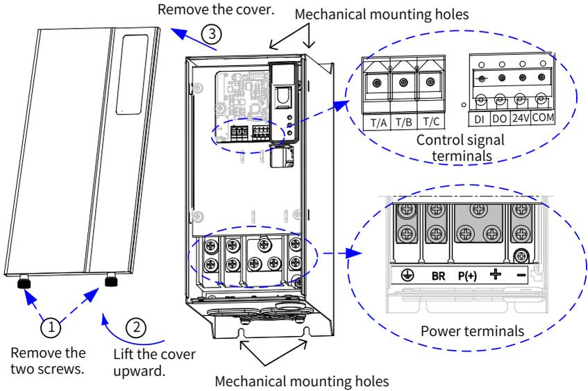
Figure 2-4 Terminals of the MDBUN series braking units (MDBUN-45-2T to MDBUN-90-2T, MDBUN-45-T to MDBUN-90-T, MDBUN-45-5T to MDBUN-90-5T)
