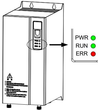
Figure 3-1 Indicators of the braking unit
