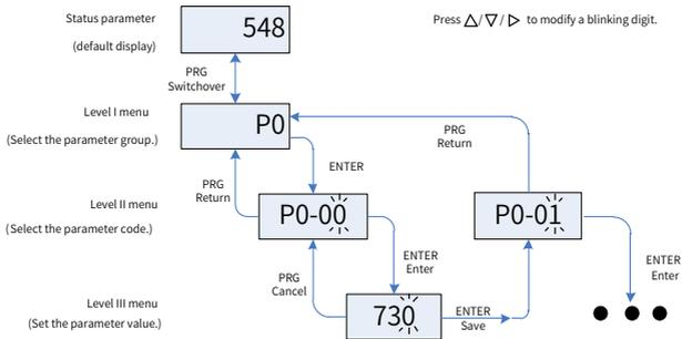
Figure 3-4 Operation procedure of the three-level menu
