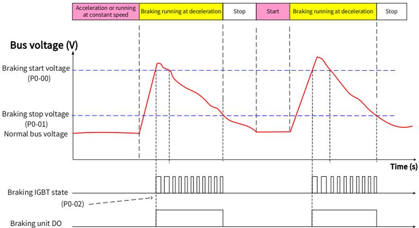
Figure 2-1 Working principle of the MDBUN braking unit
