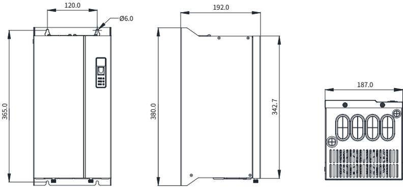
Figure 2-2 Outline dimensions (unit: mm) of the MDBUN series braking units (MDBUN-200-T, MDBUN-200-5T, MDBUN-200-7T)
