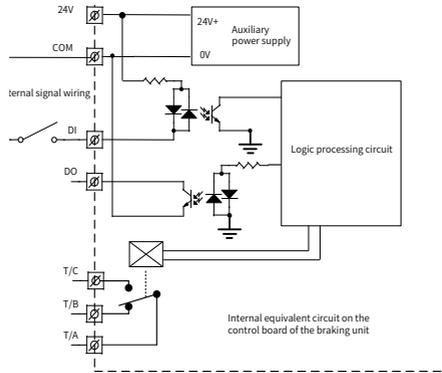
Figure 2-6 Internal equivalent circuit of the control signal terminal
