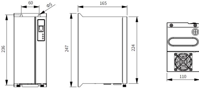
Figure 2-1 Outline dimensions (unit: mm) of the MDBUN series braking units (MDBUN-45-2T to MDBUN-90-2T, MDBUN-45-T to MDBUN-90-T, MDBUN-45-5T to MDBUN-90-5T)
