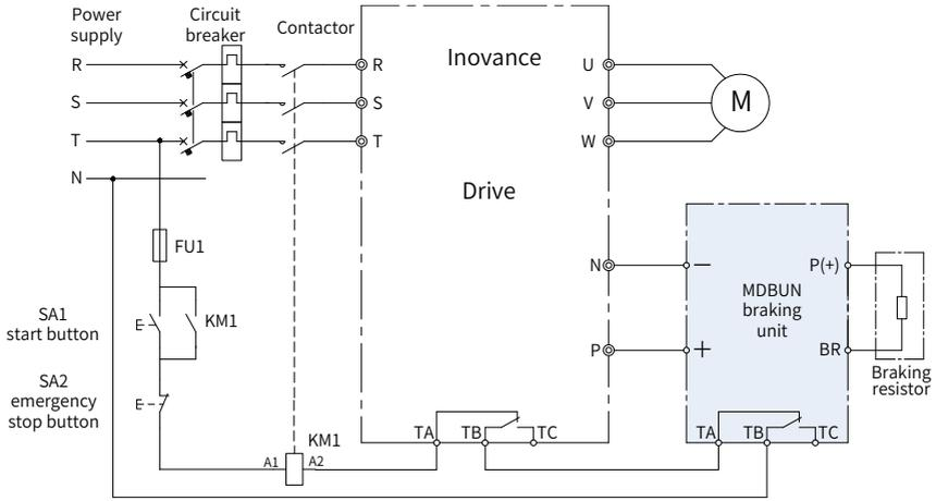
Figure 2-7 Standard wiring method 1
