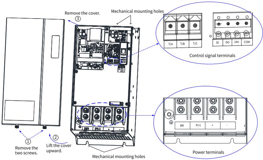
Figure 2-5 Terminals of the MDBUN series braking units (MDBUN-200-T, MDBUN-200-5T, MDBUN-200-7T)
